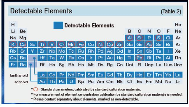
Uses X-ray fluorescence (Element analyzer) and Beta-ray attenuation (Mass) to provide continuous, in-field analysis of particulate matter (PM) concentrations and elemental composition.
