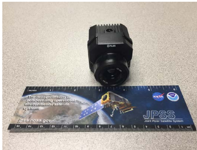
Payload #2: Infrared camera (FLIR Vue Pro R)
