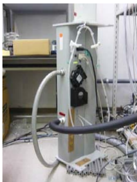
Integrating Nephelometer TSI model 3563
