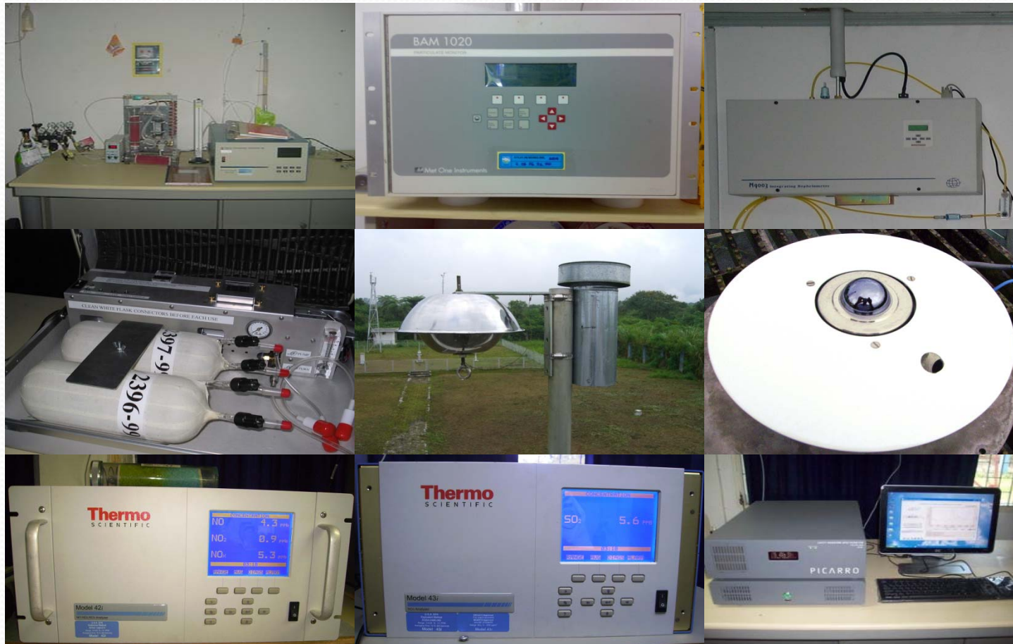
Carbon Monoxide • PM 10 mass concentration • aerosol scattering coefficient • GHGs flask sampler • POPs sampler • Pyrgeometer • NO x analyzer • SO 2 analyzer • CO 2 /CH 4 analyzer
