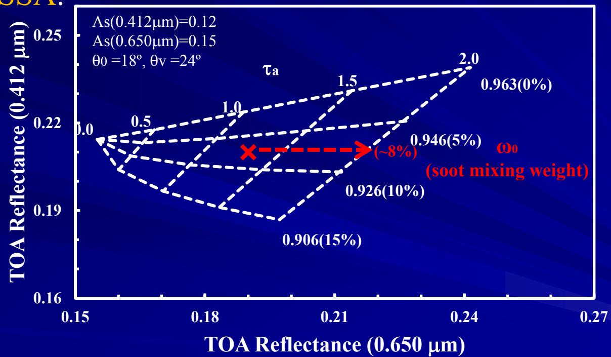
Simulated TOA reflectance as a function of AOD and SSA(mixing weights) for 412 versus 650nm channel when REFI of dust particle is 0.002.
