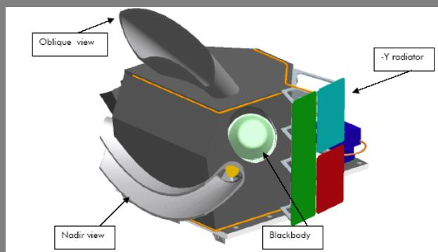
**Conical imaging radiometer with a dual view capability:**
